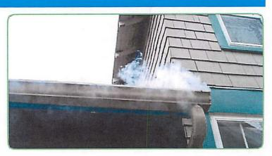
The City of Leavenworth is continuing efforts to repair the city's aging sanitary sewer system. In the next several months, customers may notice smoke coming from their sanitary sewers. This is part of a test to find leaks in the system. The nontoxic, odorless smoke is blown into sewer manholes, goes through the pipes and comes out where there are broken pipes and where roof downspouts, outside area drains, or foundation drains are connected to the sanitary sewers.
