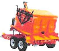
Heat Retention: Triple Wall Construction with high efficiency insulation
